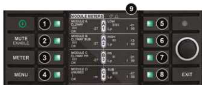
Figure 7.12: Meter Mode > Module Meters View
