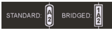
Figure 7.8: Standard and Bridge Mode Front Panel Icons (only for PLM 12K44 and PLM 20K44)
