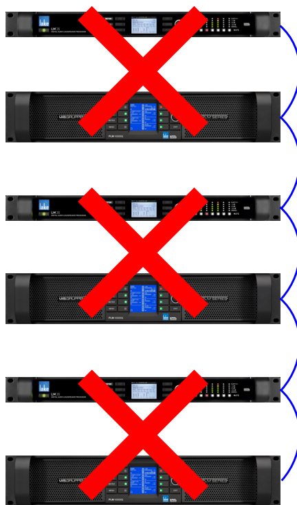
Figure 3-16: Do not daisy chain more than two Lake devices when using Dante
