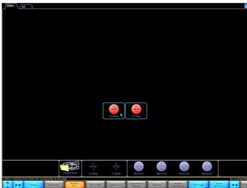
Figure 4-10: LM 26 Frame Placed in Main Work area
