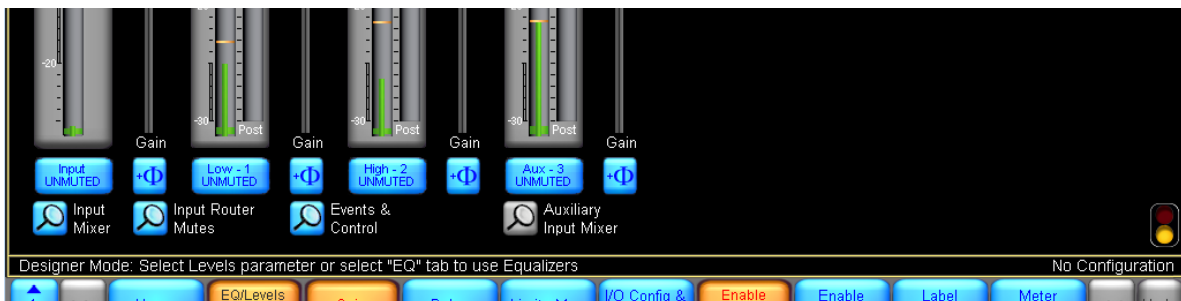
Figure 17-5: Faults and Warnings Indication via Levels screen
