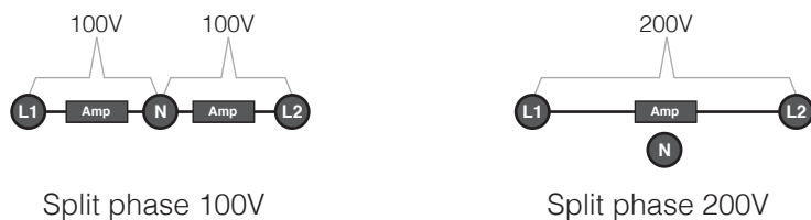
Figure 6:5: Two phase split-phase configuration
