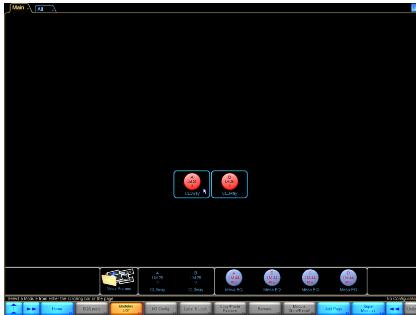
Figure 4-12: LM 26 Frame Placed in Main Work area
