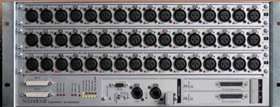
Figure 2, 48 Mic/Line Inputs, with 16 line outputs (optional)
