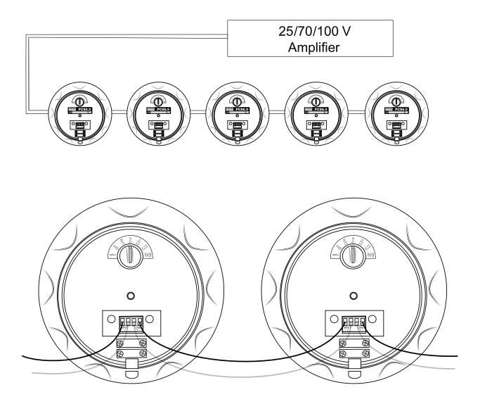
NOTE: The above example shows a total of five speakers. Using the 10W setting, you will need an amplifier with at least  $5 \times 10 \text{ W} = 50 \text{ W}$ . A good rule of thumb to remember is that the total number of speakers multiplied by the setting you select, cannot exceed the output power of the 25/70/100 V amplifier. You should select an amplifier with 20% greater power; in this example you would need an amplifier that delivers about 60 W.
