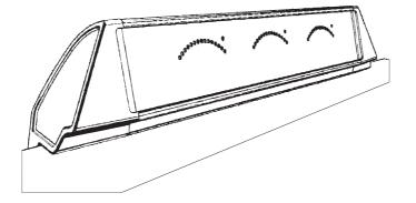
When the claws are located in the holes tip the meter bridge back to its upright position. Ensure that the ribbon cable hasn't been trapped. See Fig.3.
