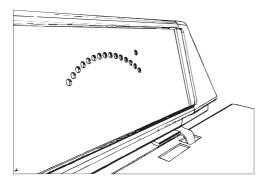
Plug the ribbon cables connector into the matching connector on the GB8. The connectors are shaped so that you cannot connect them the wrong way round. Ensure that the connectors are firmly pushed together so that the contacts are correctly seated.
