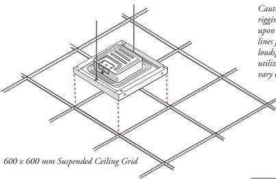
Caution: Installation must be done by qualified persons using safe rigging standards. Suspended ceiling grids can usually not be relied upon as sole support for loudspeaker. Diagram shows two support lines from suspension safety-attachment tabs on back baffle of loudspeaker. Four holes located near corners of frame can be utilized instead or in addition. Safety installation requirements vary by region. Consult a qualified installation professional.
