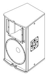
The TX1152 from Electro-Voice is a high power, high sensitivity, 2-way loudspeaker system that can be used in a variety of applications where high quality sound reinforcement is required in a lightweight package. The TX1152 utilizes the DH3, a high output 1.25 inch titanium compression driver, coupled to a Constant Directivity 60° x 40° horn. This combination results in a smooth response to 20 kHz and excellent pattern control in medium throw applications.
