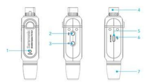
① Power and Pairing Indicator Power Functions: Flashing Red Light=Low Battery
