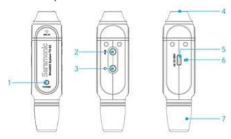
① Power and Pairing Indicator Power Functions: Flashing Red Light=Low Battery
