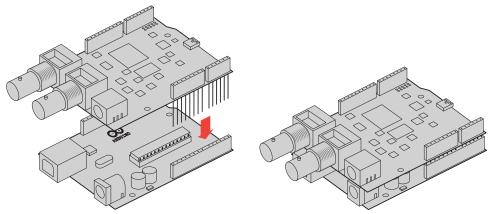
With all pins plugged in, the connection between the Blackmagic shield and the Arduino board should be firm and stable.
