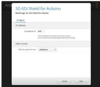
The Blackmagic Shield for Arduino Setup software lets you change settings on your shield such as the I<sup>2</sup>C address and video output format.
