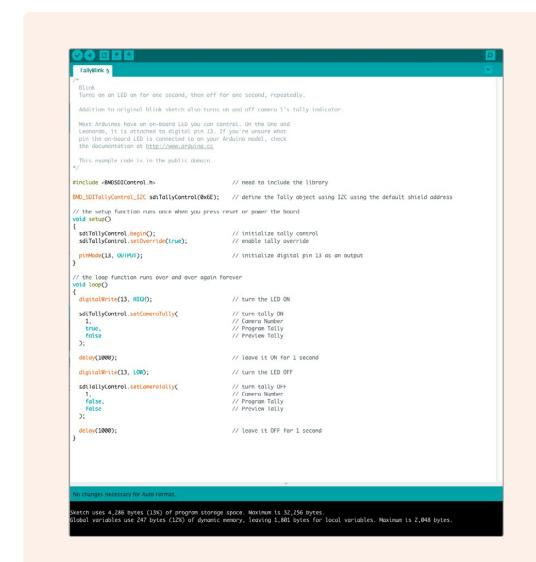
The Tally Blink example sketch is a fast and easy way to test your Blackmagic 3G-SDI Shield for Arduino. Raw data can be sent to your shield via I<sup>2</sup>C using commands from the Studio Camera Protocol document, but we have also provided custom libraries to make programming sketches much easier.
