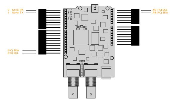
**NOTE** When connecting to the shield, communication is via  $I^2C$  or Serial. We recommend  $I^2C$  as this enables the serial monitor to be used and makes all other pins available. Select the communication mode when defining the BMDSDIControl object in the sketch. Refer to the 'Communicating with your Blackmagic 3G-SDI Shield for Arduino' section for more information.
