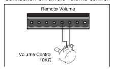
\*Note: Negative terminal should not be grounded. Never connect it to the unit's chassis or other circuit ground.
