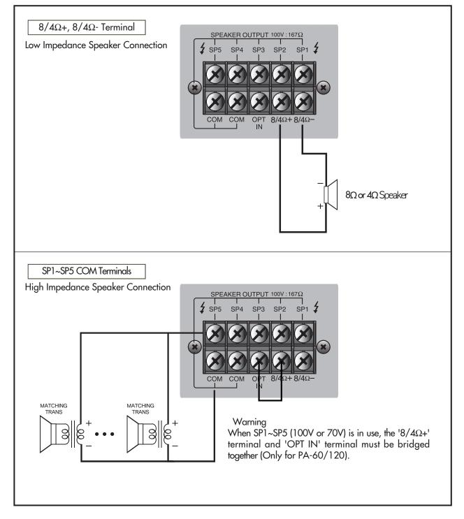
\* Warning : For high impedance systems, connect with matching transformer as the following Figure. Be certain that the total impedance is not less than the rated impedance.
