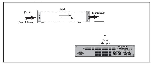
2. When using power amplifier, please install the unit where there is no airflow block to the heat sink.
