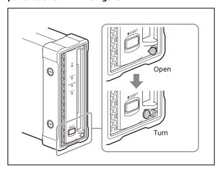
3 Insert a Phillips screwdriver 4 mm or less in diameter or the like straight in the hole.
