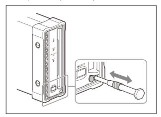
After ejecting the disc, it is not necessary to return the lever to its original position. The next time the unit is powered on, normal operation will resume.
