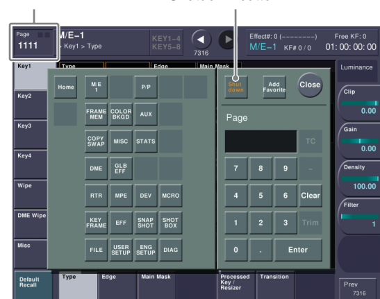
MVS-6520/3000A/3000 screen shown. On the MVS-6530, the [M/E2] button is also displayed.
