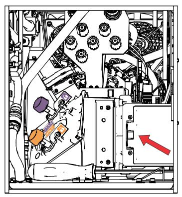
5. Loosen the lock screw for the Zoom and Focus paddles.
