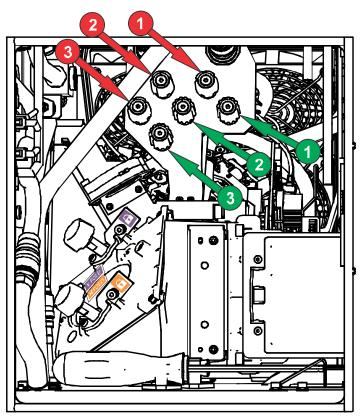
6. Use the Convergence test pattern to assist with adjusting the horizontal and vertical lines. Horizontal adjustments are controlled by adjusting knob 3.
