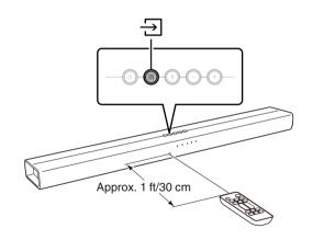
Point the remote control of the TV at the remote control sensor of this unit and press the remote control button to be learned (e.g. the button to increase the volume) once.
