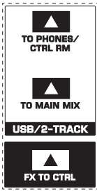
Fig. 2.12: Assignment switches of the main section
