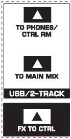
Fig. 2.12: Assignment switches of the main section
