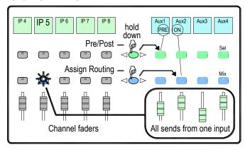
Press an Input Channel strip Mix key.
