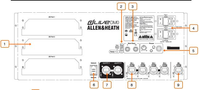
**I/O Ports** – 3x audio interface ports 128x128 channels each, independently assigned. Fit one of the option cards available for system expansion, digital mic splitting, recording or distributed audio networking. Refer to <u>www.allen-heath.com</u> for a list of available option cards.
