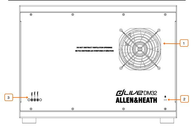
**Fan** – Ultra-quiet fan. Make sure the ventilation opening is not obstructed.
