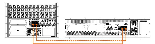
Switch on the Surface. The gigaACE Lnk/Err indicators flash at a steady rate when the link is established. The red error indicator lights if a communication error is detected. Check that the cables are correctly plugged in and are not faulty.
