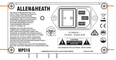
(1) dLive MixRacks ship with one PSU fitted. A second PSU can be fitted for redundancy (part number MPS-16). Loosen the 4 captive thumb screws securing the blank panel\*, slide the PSU into the slot, and tighten the 4 captive thumb screws indicated above. The MixRack will automatically switch between the supplies without interruption to the audio should one fail.
