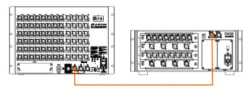
Switch on the DX Expander. The DX port Lnk/Err indicators flash at a steady rate when the link is established. The red error indicator lights if a communication error is detected. Check that the cables are correctly plugged in and are not faulty.
