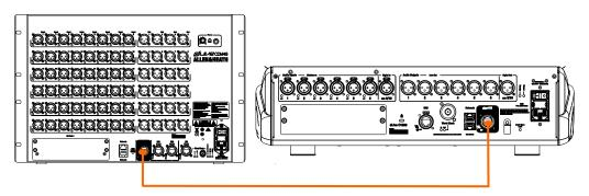
Switch on the Surface. The gigaACE Lnk/Err indicators flash at a steady rate when the link is established. The red error indicator lights if a communication error is detected. Check that the cables are correctly plugged in and are not faulty.
