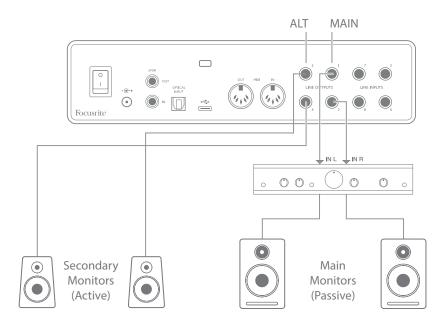
Note that as you switch between MAIN and ALT, the Line Outputs feeding the pair of speakers not in use are muted. When **speaker Switching** is disabled, Line Outputs 1 to 4 are all initially muted (for safety); you will need to unmute the appropriate outputs in Focusrite Control. Please see the Focusrite Control manual for more details of Speaker Switching.
