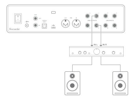
All the line output connectors are 3-pole (TRS) ¼" (6.35 mm) jack sockets, and are electronically balanced. Typical consumer (hi-fi) amplifiers and small powered monitors will probably have unbalanced inputs, either on phono (RCA) sockets, or via a 3.5 mm 3-pole jack plug intended for direct connection to a computer. In either case, use a suitable connecting cable with jack plugs at one end.
