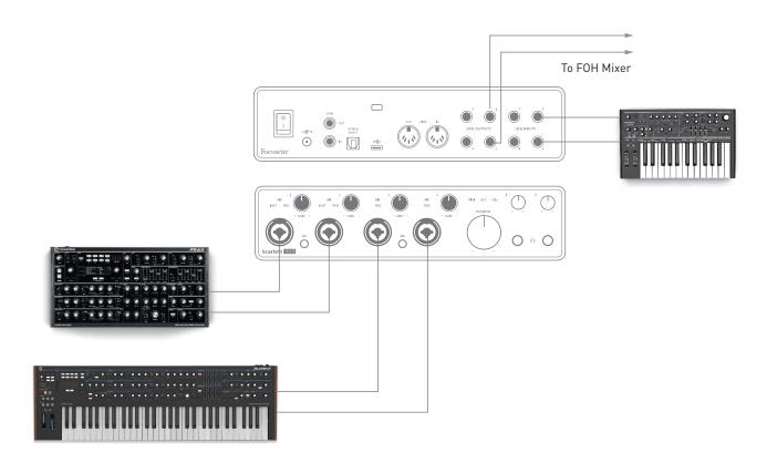
In the example illustrated, three stereo keyboards are connected to the inputs of the Scarlett 18i8; the Monitor Outputs go to the main PA system. The performer can adjust the gain for two of the keyboards against the third from the front panel; he/she can also adjust the overall level of the keyboard mix.
