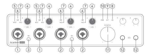
The front panel includes input connectors for Mic, Line and Instrument signals, the input gain and monitoring controls, and headphones sockets.
