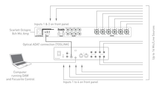
The Scarlett OctoPre's ADAT output is connected to the Scarlett 18i8's ADAT input with a single TOSLINK optical cable. To synchronise the devices, set the clock source of the Scarlett OctoPre to **Internal** and that of the Scarlett 18i8 (via Focusrite Control) to **ADAT**.
