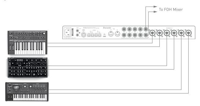
In the example illustrated, three stereo keyboards are connected to the rear panel inputs of the Scarlett 18i20; Outputs 3 and 4 go to the main PA system. The performer can adjust the gain for the individual keyboards from the front panel; he/she can also adjust the overall level of the keyboard mix.
