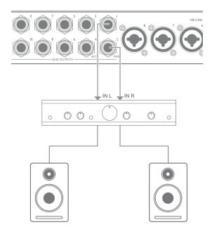
All the line output connectors are 3-pole (TRS) ¼" (6.35 mm) jack sockets, and are electronically balanced. Typical consumer (hi-fi) amplifiers and small powered monitors will probably have unbalanced inputs, either on phono (RCA) sockets, or via a 3.5 mm 3-pole jack plug intended for direct connection to a computer. In either case, use a suitable connecting cable with jack plugs at one end.
