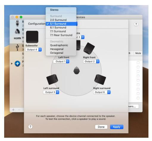
The example below shows how you would connect the six loudspeakers in a 5.1 surround monitoring arrangement.
