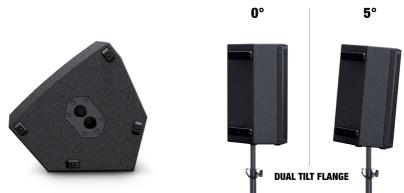
The speakers have a stand flange with a  $0^{\circ}$  angle socket (rear position) and a socket with a  $5^{\circ}$  tilt angle (front position). Examples of use: Use the socket with the  $0^{\circ}$  angle for standing audiences and the socket with the  $5^{\circ}$  tilt angle for seated audiences.
