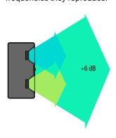
The combined signal of the two relatively small drivers propagates forward like a single waveform, behaving like a single, larger driver. This mutual coupling provides a highly dynamic output in a compact footprint. At the same time, the two smaller woofers work in parallel to partially contain the dispersion of the tweeter, minimizing phase
