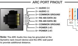
The Symetrix ARC-PSe provides serial control and power distribution over standard CAT5/6 cable for systems with more than 4 ARCs, or, when any number of ARCs are located long distances from a Integrator Series, Jupiter or Symetrix DSP unit.
