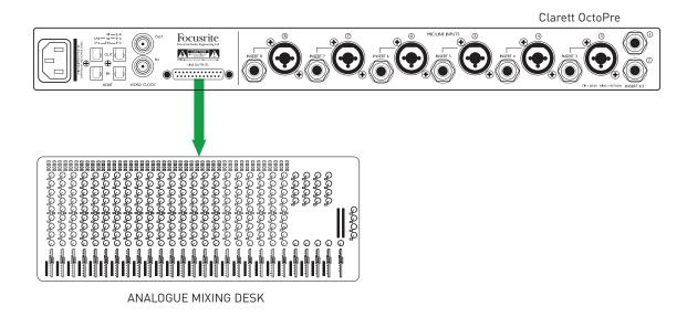
This setup uses the Clarett OctoPre's mic pre-amplifiers and AIR mode to provide a high quality "front end" for an analogue mixing desk. Use an 8-way loom to connect the OctoPre's **LINE OUT**
