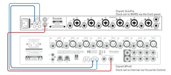
This example shows the same setup as Example 2, but running at a sample rate of 96 kHz ("SMUX-II" mode). Both units must be set to 96kHz; two optical cables are used, carrying four channels of audio each. The Clarett 8PreX is the sync master as before.
