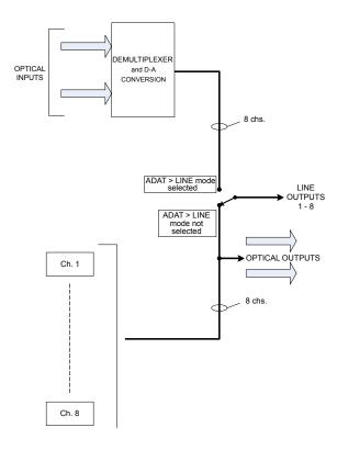
This mode enables the Clarett OctoPre be used to connect an 8-channel ADAT format output (from a DAW, for example) to a set of analogue inputs, typically the channels of an analogue mixing console, to permit such a mixer to be used to mix down DAW tracks.
