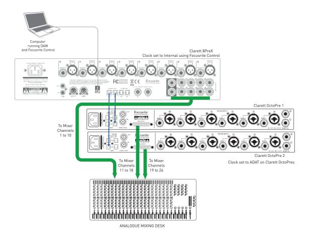
This example shows how to connect a greater number of DAW tracks to an analogue mixing desk for mixdown. The 10 analogue outputs of a Clarett 8PreX interface are connected to desk Channels 1 to 10. Its **OPTICAL OUT** ports are connected to the **OPTICAL IN** ports of two Clarett OctoPres with ADAT > LINE mode selected on both. A loom similar to that used in Example 4 is then used to connect the two OctoPres to Channels 11 to 26 of the desk.
