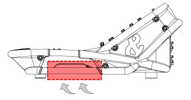
Leave adequate space for ventilation ( $\checkmark$ ) at the sides of the mixer in the area indicated.
