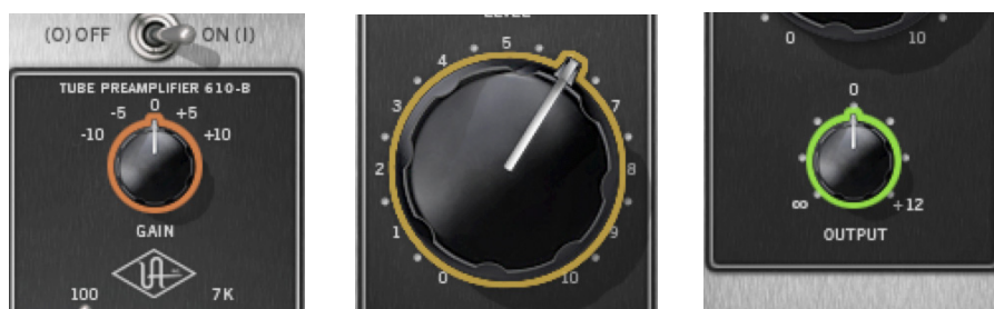
The matching color outline on the parameter in the Unison plug-in interface indicates which gain stage is being controlled by Apollo's front panel preamp knob
