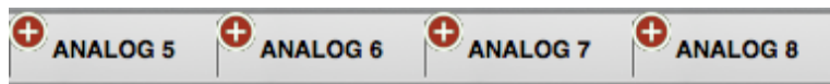
The PASTE modifier appears on input names after copying a channel strip
