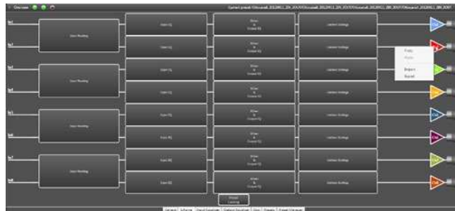
FIGURE 43: All possible channel operations are available by right clicking on the respective channel.
