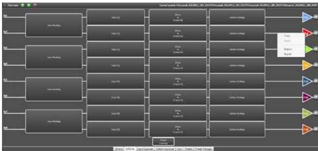
FIGURE 54: All possible channel operations are available by right clicking on the corresponding channel.
