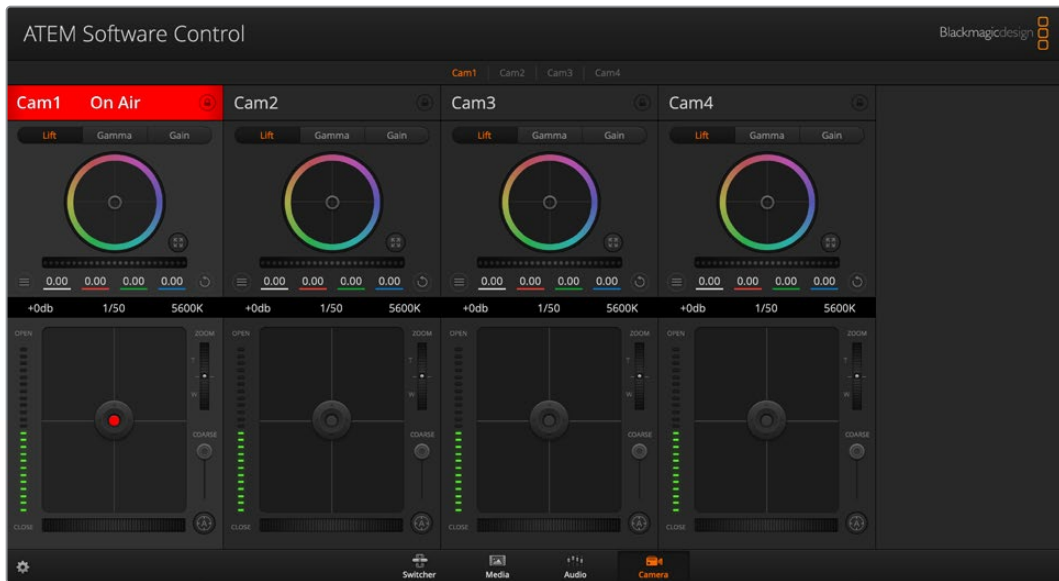
Camera control lets you control Blackmagic Pocket Cinema Camera 4K and 6K with ATEM Mini
