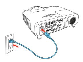
Press the (1) power button on the projector or remote control. The projector beeps, and the Status light flashes blue and then stays on.
