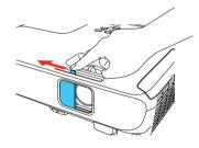
4 Press the power button on the projector or remote control. The projector beeps, the Status light flashes blue, and then stays on.
