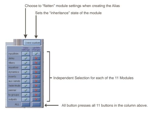
Copy Settings Column: When a custom Alias is created, a tick indicates the new Alias will keep the current channel settings for the given module.
