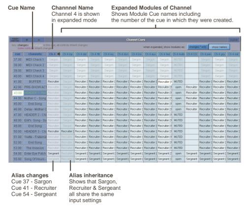
NOTE: When Channel Cue information is expanded to show individual modules, busses that are bigger than Mono (Stereo and Surround) display one column for each of the legs of the buss (eg separate Left and Right legs in stereo)
