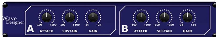
**WAVE DESIGNER** is a powerful tool for adjusting signal transients and dynamics such as attack and sustain. Use it to make a snare drum really "crack" in the mix or level out volume inconsistencies of slap bass tracks. (Inspired by SPL Transient Designer\*)
