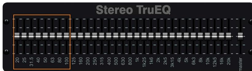
Unlike typical graphic EQs, our **STEREO TruEQ** delivers the exact frequency response for the new fader setting, taking neighboring fader settings into account – for surgical and responsive filtering or general room equalization (Modeled after BEHRINGER UltraCurve DEQ2496). The MR18 can provide up to 16 mono graphic EQs – one in each of the 6 Aux Buses and Main LR, plus 8 additional mono GEQ effects (4 stereo) that may be inserted into channels.
