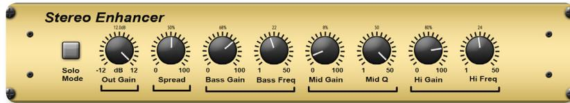
**ENHANCERS** let you emphasize the Bass, Midrange and Hi output at selectable frequencies, allowing you to generate maximum punch, clarity and detail – without turning up the overall volume. (Inspired by SPL Vitalizer\*)
