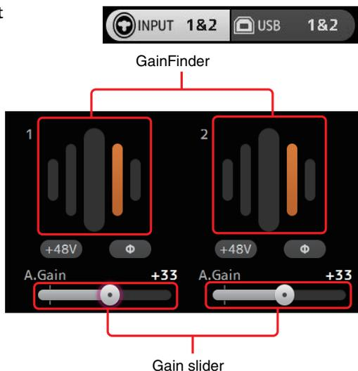
5. Touch the digital gain text box to highlight it, then use the [TOUCH AND TURN] knob to adjust the setting.
