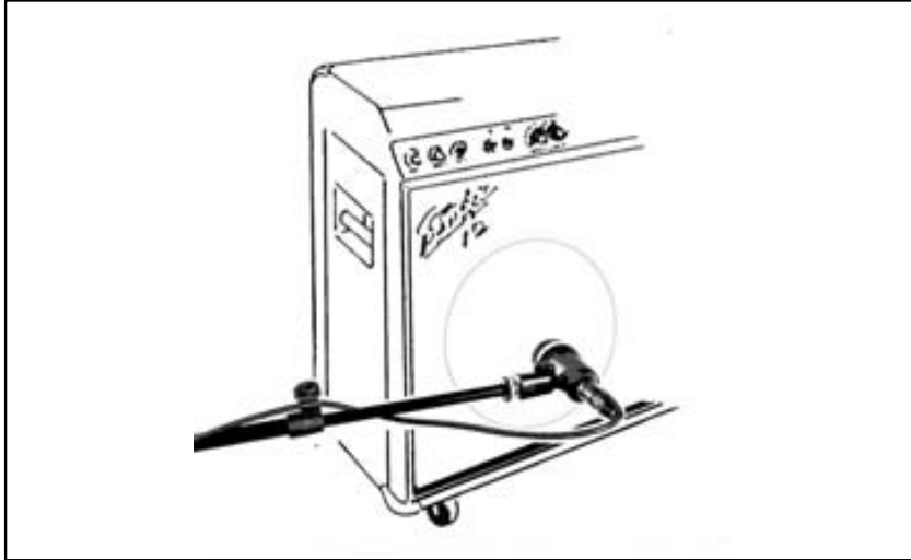
Fig. 3: Microphone placement for a guitar amp.
